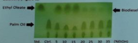
Figure 2. Effect of % ethanol in biodiesel reaction at 1 h analyzed by Thin Layer Chromatography
